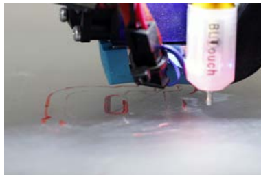
Extruder is too low and digging into bed
