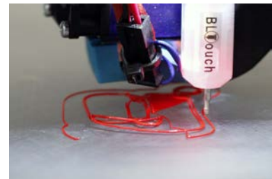
Extruder is too high and printing in air
